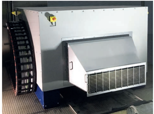
Fahrtwind-Simulator type VQF 800/1250, height-adjustable, extensible air outlet nozzle
