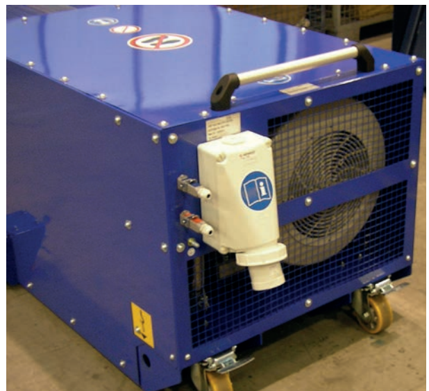
Fahrtwind-Simulator type VQF 500/800 for vehicle roller type dynamometers, drive side with electrical connections.
